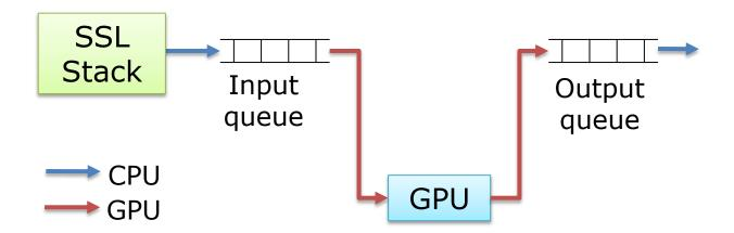
Batch size is dynamically adjusted to queue length
